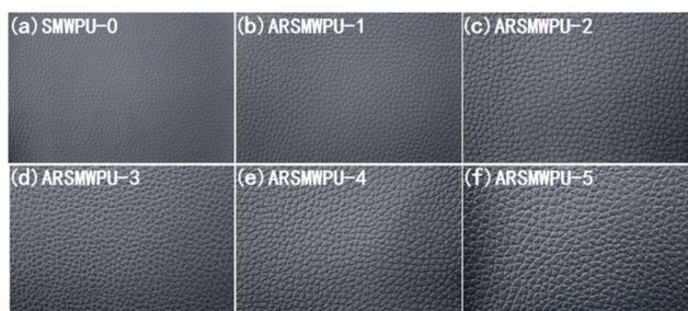
Fig. 10 Effect of different polysiloxane contents modifying self-mattting WPU on gloss of the leather coating.
