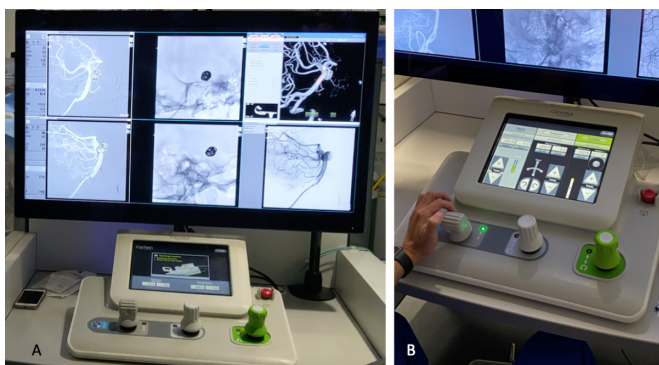
Figure 3 The operator's perspective. (A) The screen and the control console. The robotic arm is operated using three joysticks: one for microcatheter, one for microwire and one for the devices (stent and coils). (B) Closer view of the control console showing the screen during coil placement. The small screen shows three columns, each corresponding to a joystick, with additional commands such as millimetric moves for the microcatheter and devices or predefined rotations for the microwires.
