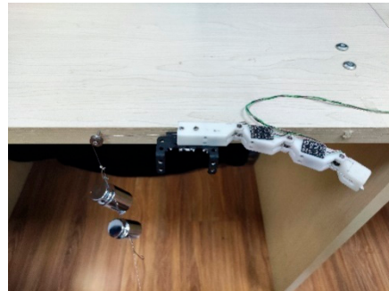
Figure 15. Experimental setup for evaluating the relationship between driving force and finger bending angle.
