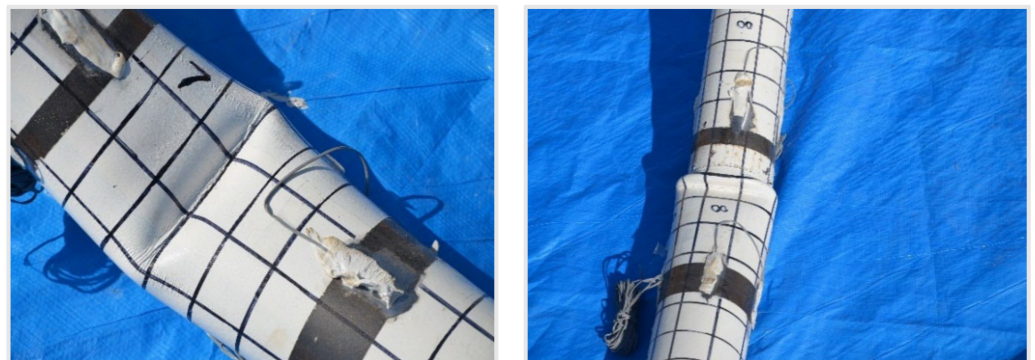
Figure 22. Cross-section ovalization of specimens BT7 (kink) and BT8 (fold).
