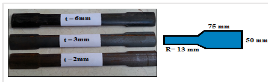
Figure 2. Tensile specimen dimensions.
