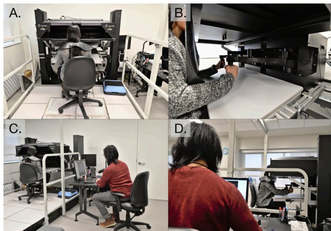
Figure 2 Photos of the Kinarm robotic system set-up. (A) Patient will be seated in front of the robot so that they are able to view the horizontal screen. (B) Using the robot's handles, patients will complete eight standardised tasks measuring cognitive, sensory and motor function. (C) and (D) A trained research associate will lead the assessment session. Photos are used with permission.
