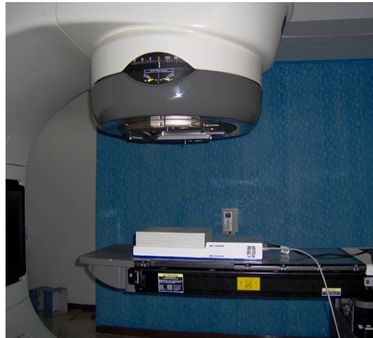
Fig. 1. Measurement setup at the accelerator with I'matriXX.
