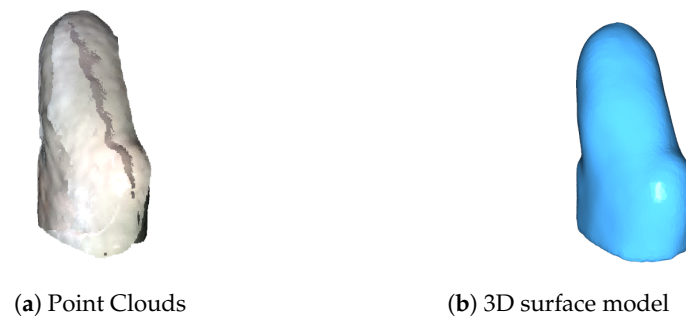
Figure 12. Comparison of (a) the initial global 5 images alignment and (b) the output model after applying a refined ICP registration and Poisson surface reconstruction. This shows the input and the output of the reconstruction algorithms.
