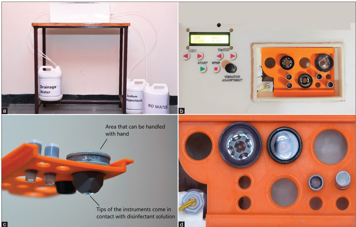
Figure 1: (a) Semiautomated lens disinfection unit, (b) Main unit with display, (c and d) Instrument tray for contact lenses
