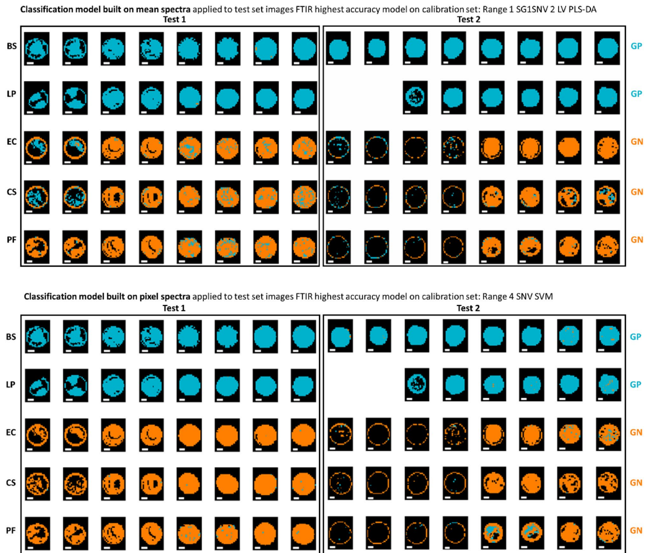
Figure 4. Classification maps for samples in the test sets obtained from the best mean (top panel) and pixel-level (bottom panel) FTIR models for GP/GN classification. Pixels classified as GP/GN are shown in blue or orange respectively. Each replicate has two drops. BS: Bacillus subtilis ; LP: Lactobacillus plantarum ; EC: Escherichia coli , CS: Cronobacter sakazakii ; PF: Pseudomonas fluorescens . White scalebar indicates 1 mm (width) × 0.2 mm (height).
