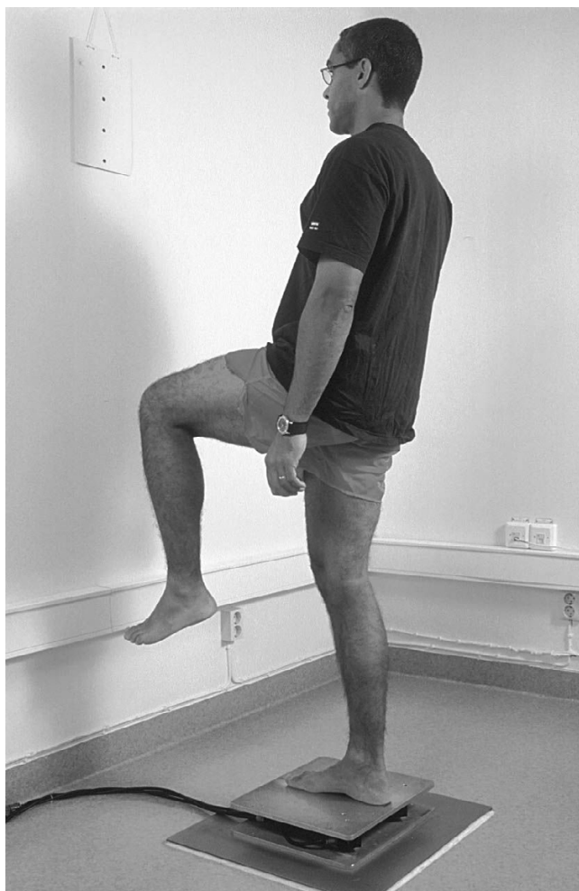
Figure 1 Stabilometry in single-limb stance, tested by means of a strain gauge force plate. A standardized position was used. The subject is a model who did not participate in the study. Reprinted from Ageberg E, Zätterström R, Moritz U, Fridén T. Influence of supervised and nonsupervised training on postural control after an acute anterior cruciate ligament rupture: A 3-year longitudinal prospective study. Journal of Orthopaedic & Sports Physical Therapy . 2001;31: 632–644, with permission of the Orthopaedic and Sports Sections of the American Physical Therapy Association.
