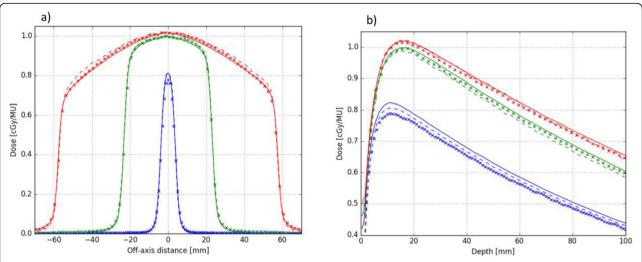
**Fig. 2** Dose profiles (a) along MLC leaf travel direction and depth dose curves (b) for microDiamond measurements (solid), Precision MC (dashed) and IDC (symbols) for 7.6 mm × 7.7 mm (blue), 46.2 mm × 46.2 mm (green) and 115.0 mm × 100.1 mm (red) rectangular MLC fields in water
