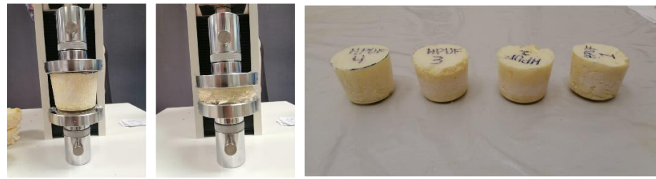
Figure 6. Prepared samples of closed-cell hydrophobic polyurethane foam (HPUF) with various densities and the compression test setup.
