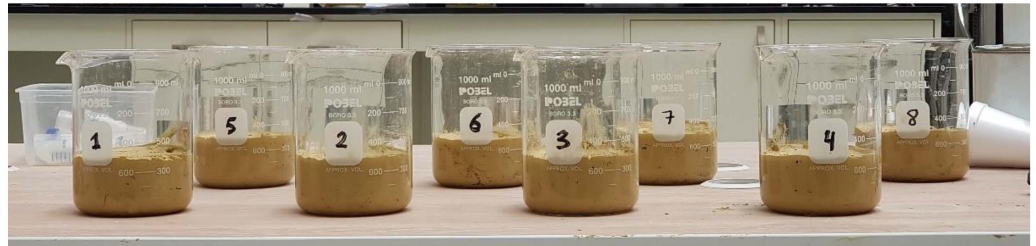
Figure 5. Large-scale free swell arrangement prepared to test Na-bentonite specimens in wet-shrink cycles.
