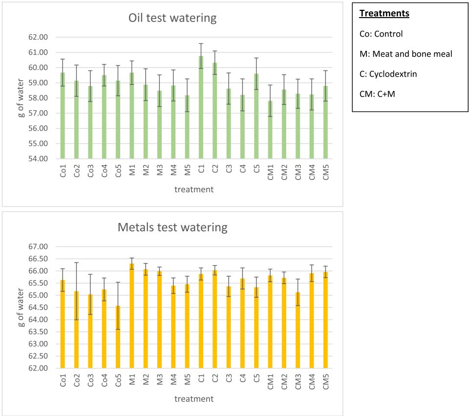
Fig. 1. Average amount of water, in grams, contained in each treatment during the experiment, and the related fluctuations in time ( \pm SD). The amount of water contained in each beaker was kept at around 60% of the WHC.
