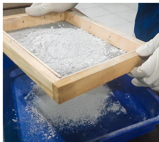
Figure 2. Filtering ground glass with a filter with a mesh size of 200.
