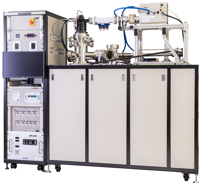
Figure 4. An example of a top-hat MWCVD reactor (Seki model SDS6380). This reactor has power supplies up to 5 kW (at 2.45 GHz) and is capable of depositing polycrystalline diamond films, SCD diamond plates or SCD gemstones at high rates. The chamber is water-cooled, with a substrate platen capable of accommodating samples up to 50 mm in diameter. Photo courtesy of Philippe Bergonzo, Seki Diamond Systems [13].
