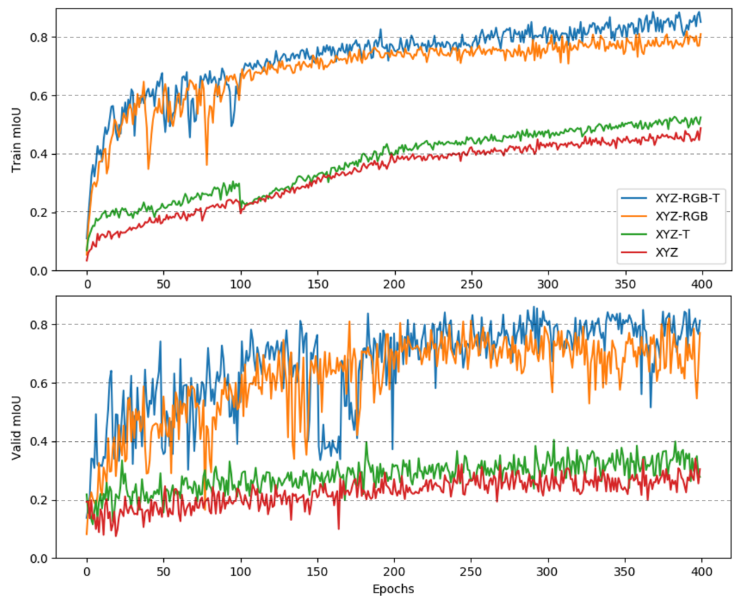
Figure 8. The convergence curves in training phase of RandLA-Net, in which RandLA-Net was trained for 400 epochs on data XYZ, XYZ-T, XYZ-RGB, and XYZ-RGB-T. Upper—the training curve; bottom—the validation curve.
