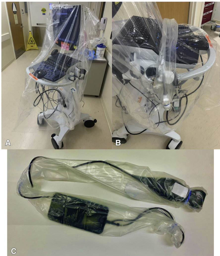
Figure 6. Large plastic equipment cover over POCUS cart-based machine (A) with disposable ultrasound probe over phased-array ultrasound probe (B). Disposable ultrasound probe cover encompassing the entirety of a hand-held portable ultrasound (C).
