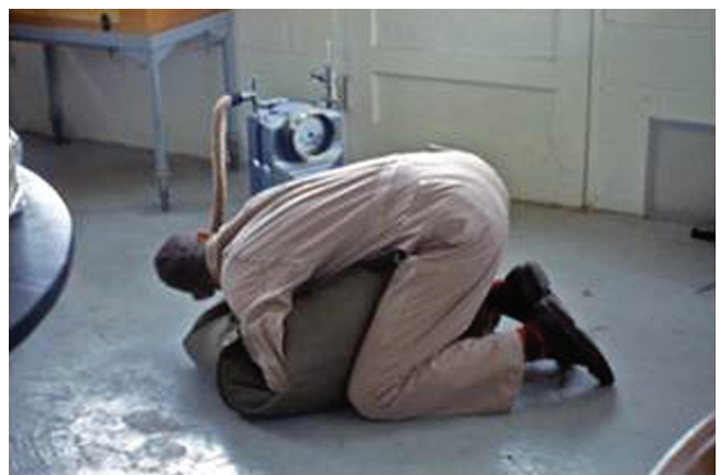
Figure 7: Jack with bag of expired air being pushed through gas meter to measure volume.
