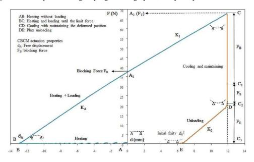
**Figure 3.** Example of fixing or programming cycle, fixity temperature  $T_{\rm F} = 150$  °C.
