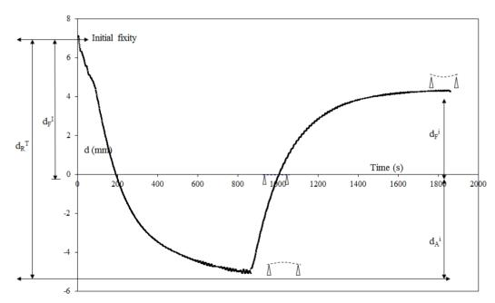
To study the evolution of deformations during multi-step unconstrained recovery test versus  $T_R$ , the fixity ratios  $r_F$  and recovery activation ratios  $r_A$  are calculated:
