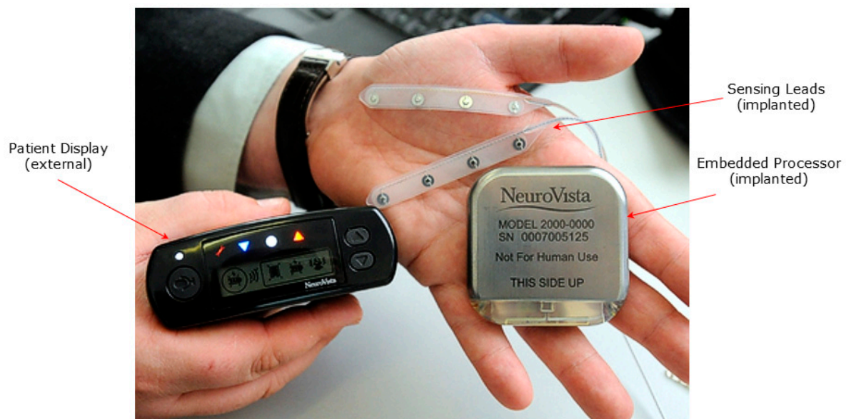
Figure 2. Seizure Advisory System (SAS) shown with implanted subdural electrodes, implanted EEG processor and telemetry unit, and external patient advisory module with red, white and blue indicator lights.
