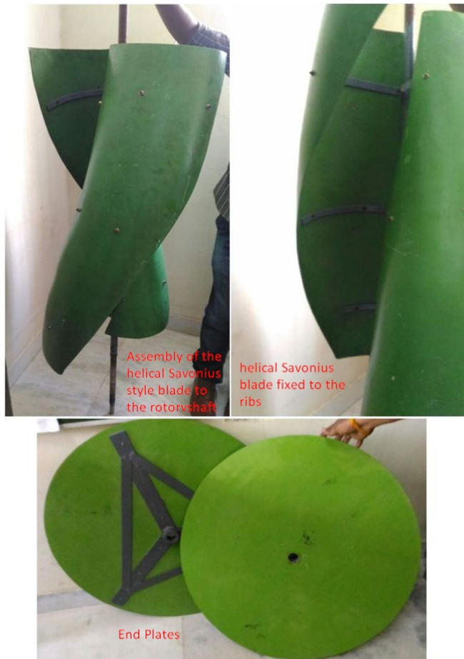
Fig. 4. Assembled helical Savonius style blade to the rotor shaft of VAWT.
