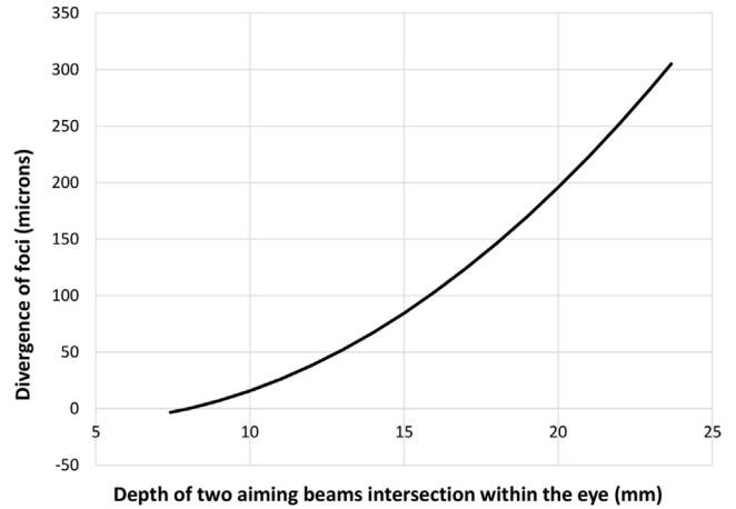
Figure 1. The graph shows the distance between the 2 focal points, neodymium-doped yttrium aluminum garnet (Nd:YAG) and its aiming beam, as a function of the depth inside the eye. As the device is moved closer to the eye, the depth of the focal points of both the Nd:YAG and of diode laser increases, while the 2 points progressively diverge from one another.
