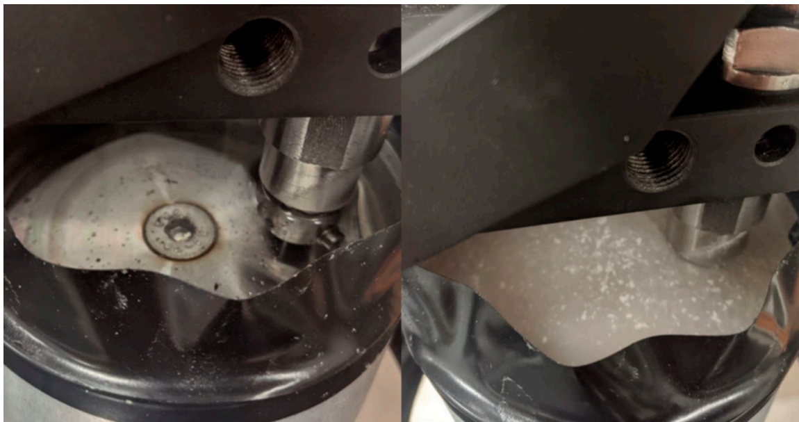
Figure 19. (Left) Water contamination with wear products after examination of the fibrous composite and (right) the unreinforced ABS polymer.
