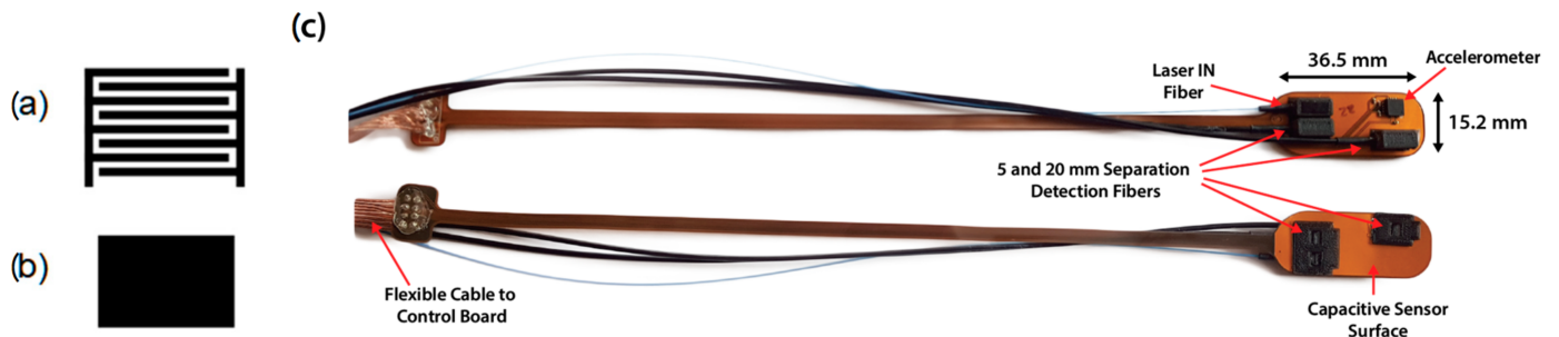
Figure 1. (a) Drawing of an interdigitated comb electrode (V1). Two comb-shaped electrically conductive electrodes are placed in an interdigitated fashion and each comb finger acts as a plate of a mutual planar capacitor with the adjacent fingers. (b) Drawing of a self-capacitance single electrode (V2), where an isolated copper plate acts as a plate of a planar capacitor. (c) Pictures of the probe flexible printed circuit board (PCB) equipped with the single-electrode contact sensor. Top—Probe top view: the accelerometer Integrated Circuit (IC) and the 3D-printed fiber holders, not in contact with the subject’s skin. Bottom—Probe bottom view: a copper plane covering the whole bottom layer of the PCB acts as single sensing electrode for the contact measurement.
