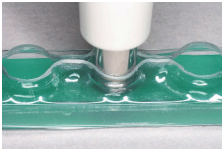
FIGURE 5: Adapter with sensor tip (Spectrophotometer VITA Easyshade, VITA Zahnfabrik, Bad Säckingen, Germany) measuring an Orthocryl green test specimen.
