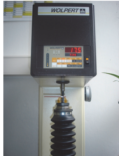
FIGURE 3: Instron Wolpert- Macro Hardness K-Testors 2524 (Wolpert Wilson Instruments, Pfungstadt, Germany) including a Forestacryl pink test specimen.
