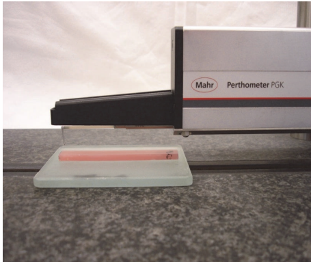
FIGURE 4: Surface measuring station Perthometer S3P (Perthometer S3P, Mahr GmbH, Göttingen, Germany) measuring a Forestacryl pink test specimen.
