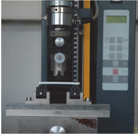
FIGURE 2: Three-point bending device on the Zwick universal testing machine (ZWICKI TMZW, Zwick GmbH & Co. KG, Ulm, Germany) and Forestacryl colourless test specimen.
