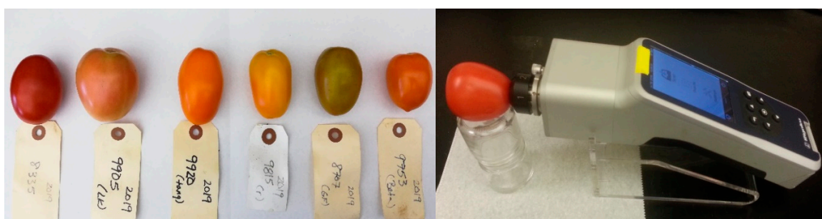
Figure 1. Tomato samples and surface scan using Rigaku's Progeny handheld Raman spectrometer.
