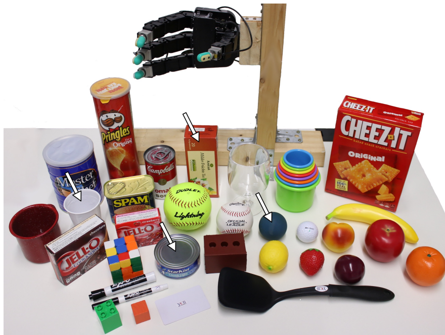
Figure 2. Test objects. Most of the objects were from the YCB object set [38] where only the tea box and the white plastic cup are not in the original set. The training set (indicated by the white arrows) included 4 objects only: a tuna can, a plastic cup, a ball, and a tea box.
