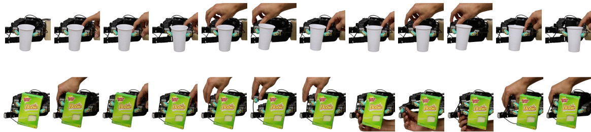
Figure 7. Experiments showcasing master–slave operation where the fingers stabilize the object despite one finger introducing perturbations to change the object’s positions in-hand. The experiment showcases how the independent finger grip stabilization controllers, paired with upper level control policies, can enable in-hand object manipulation. Instead of an upper level controller, finger perturbations were introduced by a human experimenter for a two-finger grasp (upper row) and a three-finger grasp (lower row). In addition, in the three-finger grasp we show that fingers can be removed from the object while it is re-stabilized by the remaining fingers.
