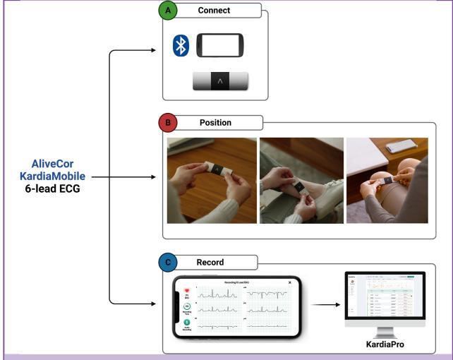
**FIGURE 1.** KardiaMobile 6L (AliveCor, Inc) ECG Recording. A, Portable ECG device is connected by Bluetooth to a smartphone or tablet with installed Kardia application. B, In the sitting position, patients place both thumbs on the anterior electrodes, while simultaneously placing the posterior electrode on the left ankle or left knee. C, Six-lead ECG of 30-second duration was recorded and automatically saved into the KardiaPro (AliveCor, Inc) portal. ECG, electrocardiography.
