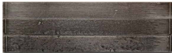
Fig. 10. Macroscopic photos of the 1# tube sample after 720 h of SSCC.
