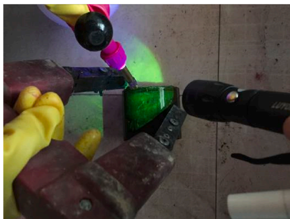
Fig. 2. Magnetic particle testing around the outer surface of the fracture tube section.
