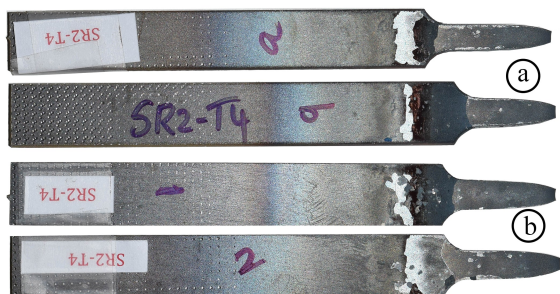
(a) Fractured specimens at 950 °C and 0.1 s -1
