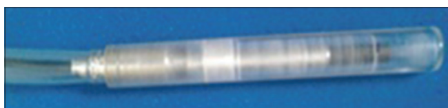
Figure 1: Locally fabricated perspex protection cap with an extended coverage till the end of aluminum stem of the ionization chamber
