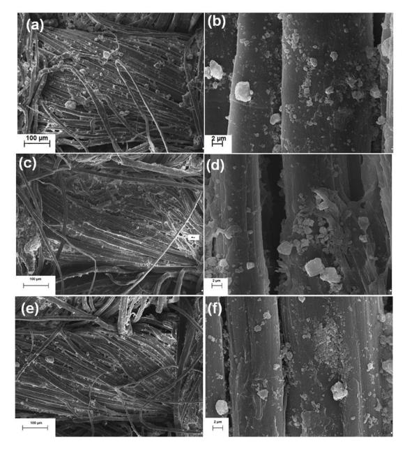
**Figure 2.** Scanning electron micrographs of: (**a**,**b**) linen woven fabric after alkaline treatment and dip-coating with 5% wt. of CuO-SiO<sub>2</sub>, (**c**,**d**) linen woven fabric after enzymatic treatment with 2.5 U/g of laccase and dip-coating with 5% wt. of CuO-SiO<sub>2</sub>, (**e**,**f**) linen woven fabric after enzymatic treatment with 5.0 U/g of laccase and dip-coating with 5% wt. of CuO-SiO<sub>2</sub>.
