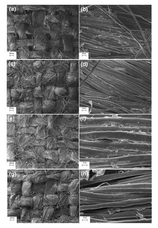
**Figure 1.** Scanning electron micrographs of: (**a**,**b**) raw linen woven fabric, (**c**,**d**) linen woven fabric after alkaline treatment, (**e**,**f**) linen woven fabric after enzymatic treatment with 2.5 U/g of laccase, (**g**,**h**) linen woven fabric after enzymatic treatment with 5.0 U/g of laccase.
