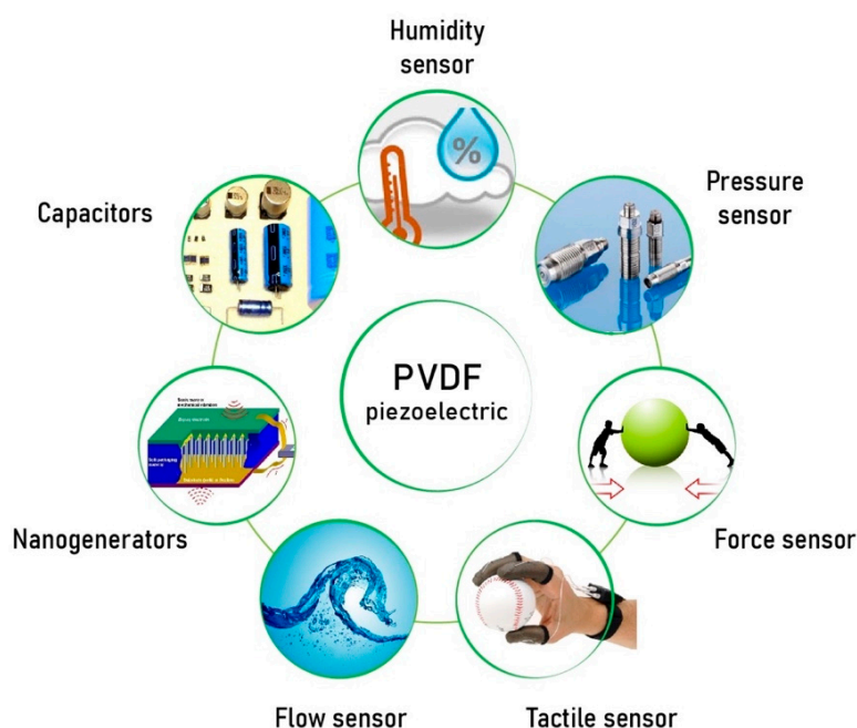
Figure 16. Applications of piezoelectric electrospun PVDF films for different devices.
