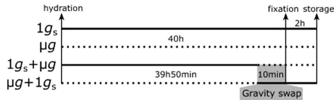
Figure 4. PolCa experimental timeline as performed in the Kubik facility. The cosmonaut positioned four experimental units (EUs) on a centrifuge and four EUs in microgravity conditions, triggering simultaneously an automatic water injection in the CCs. The water injection, leading to seed hydration, was considered as the starting point of the experiment. 39 h50 after hydration in simulated gravity, two EUs were transferred to microgravity conditions by the cosmonaut and correspond to 1g_s + \mu g samples. At the same time, the two EUs initially in microgravity were placed on the centrifuge, corresponding to \mu g + 1g_s samples. The time period of gravistimulation onset and removal corresponds to 10 minutes for each CC. Two EUs were left on the centrifuge, corresponding to control simulated gravity ( 1g_s ) and two others were kept in microgravity conditions, corresponding to control microgravity ( \mu g ). In each EU, fixative solutions were automatically injected from the pouch connected to the CC, leading to the fixation of all seedlings in their growth conditions at 40 h after hydration. EUs were left on the centrifuge or in microgravity for 2 h and then stored at 6^\circ\text{C} until being opened on Earth. The solid lines indicate the time period in simulated gravity. The dotted lines indicate the time period in microgravity.
