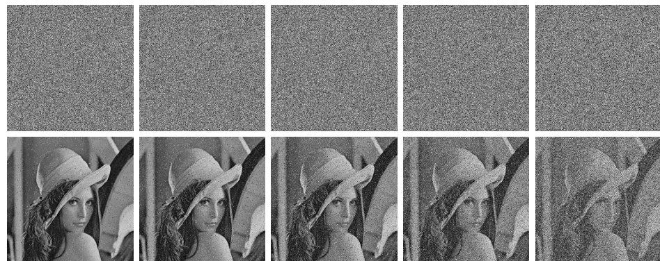
Figure 8. Noise test. The first row, from left to right: cipher images with 0.5%, 1%, 2%, 4%, and 10% salt-and-pepper noise added. The second row: the decrypted images from the corresponding cipher images in the first row.
