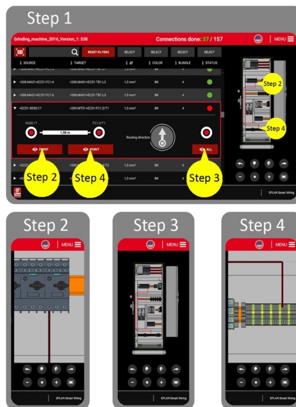
Figure 3. EPLAN Smart Wiring (ESW) application (Step 1) with 3 zooms of the 3D graphics, showing the zoomed connection point (Step 2, Step 4) or whole wiring routing (Step 1, Step 3).
