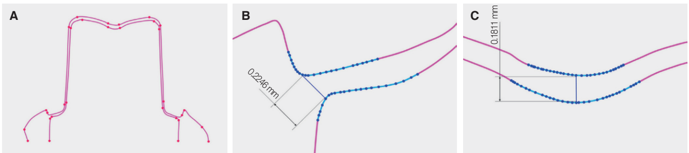
Fig. 4. Fit evaluation in computer-aided replica technique. (A) Digital sectioning of 3D image of gap space in the buccolingual plane, (B) Marginal gap measurement using a software program, (C) Occlusal gap measurement using software program.
