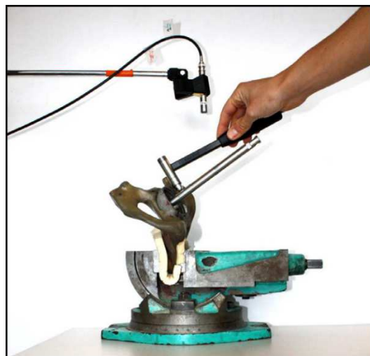
Figure 9. Example of in vitro testing of the T1-L3 technology for uncemented fixations of the acoustic approach. The following components are included; artificial pelvis, microphone (suspended above the artificial pelvis), the metal rod (connected to the acetabular cup), and the hammer (used to drive the system). Reprinted from [56] with permission from Elsevier.
