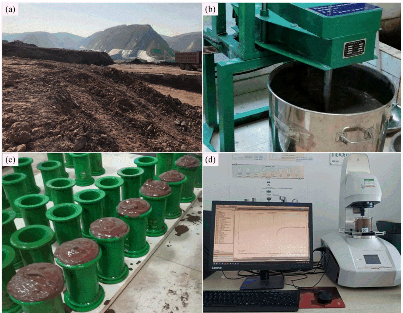
Figure 2. Tests of RMCB: (a) dry yard of BRM; (b) preparation of RMCB; (c) mixture proportion test; (d) shear rheological test.
