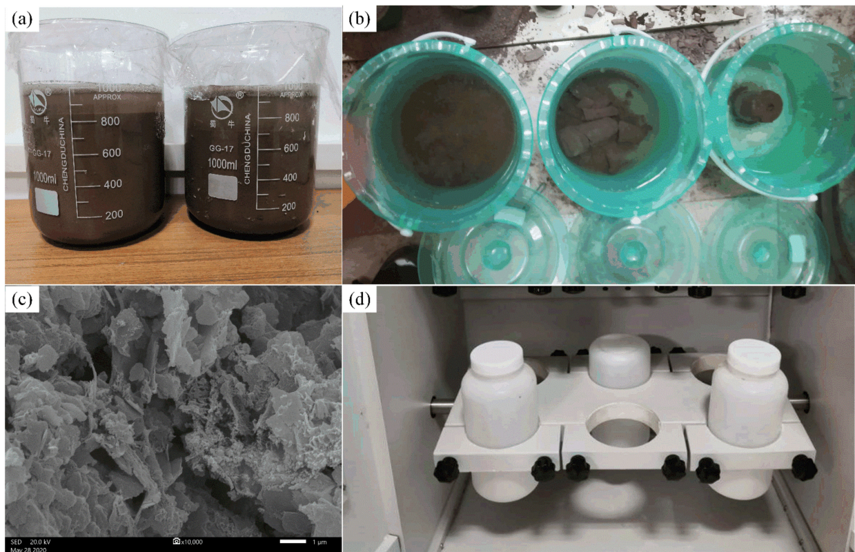
Figure 3. Contamination analysis experiments of RMCB: (a) bleeding experiment; (b) immersion experiment; (c) SEM of RMCB; (d) toxic leaching experiment.
