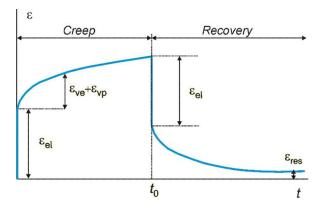
Figure 9. A schematic strain vs. time curve in a creep-recovery test.
