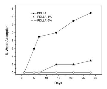
**Figure 6.** Kinetics of water absorption of poly(D,L-lactide) filled with cellulose nanowhiskers at different filler contents indicated on the graph. Reproduced with permission from [13]. Copyright © (2011). Elsevier Ltd. (licence No. 5135221438116).
