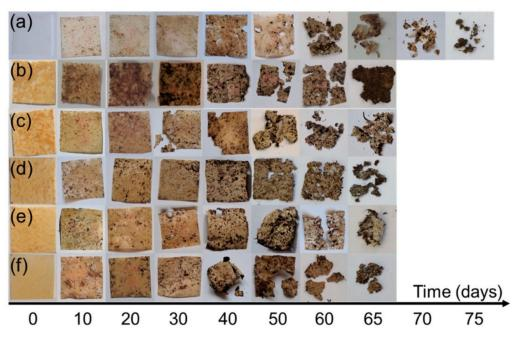
**Figure 2.** Photos of (**a**) PBS; (**b**) 40% NFC; (**c**) 7/3; (**d**) 5/5; (**e**) 3/7 and (**f**) 40% MCC films during biodegradation studies in soil burial test conducted in composting conditions [55].
