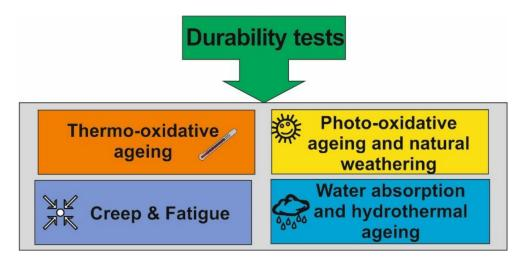
Figure 3. Basic types of durability tests for polymer composite materials.
