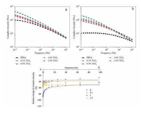
**Figure 5.** Complex viscosity of pure PBSA and PBSA/TiO<sub>2</sub> nanocomposites (**a**) before and (**b**) after 360 h of UV irradiation as a function of frequency at 140 °C (reproduced from [100], copyright © (2019). Hindawi, (**c**) relative change of complex viscosity of PBSA filled with TiO<sub>2</sub> (relative weight content is indicated on the graph) vs. frequency. Dots: experimental data used from [100]; lines: approximations by logarithmic functions.
