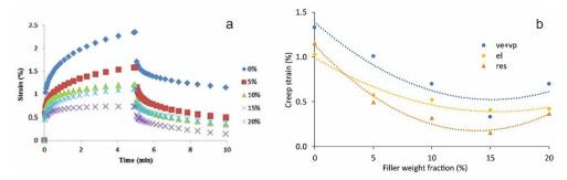
**Figure 10.** The (**a**) creep-recovery vs. time curves of starch only and starch–CNF composite films (reproduced with permission from [10], copyright © (2015), Elsevier Ltd., licence No. 5143001008321). (**b**) Viscoelastic and viscoplastic (ve+vp), elastic (el) and residual (res) strains of starch modified with cellulose nanofibrils vs. filler weight fraction. Dots: experimental data from [10]; lines: approximations by polynomial functions.
