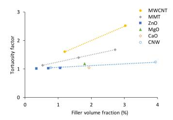
**Figure 7.** Tortuosity factor as a function of filler volume fraction for PLA filled with different nanofillers (indicated in the legend).
