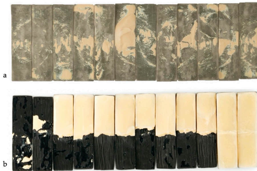
Figure 5. Specimen surface after fracture failures. (a) Metal–ceramic specimen failures; (b) carbon-fiber-reinforced composite specimen failure.
