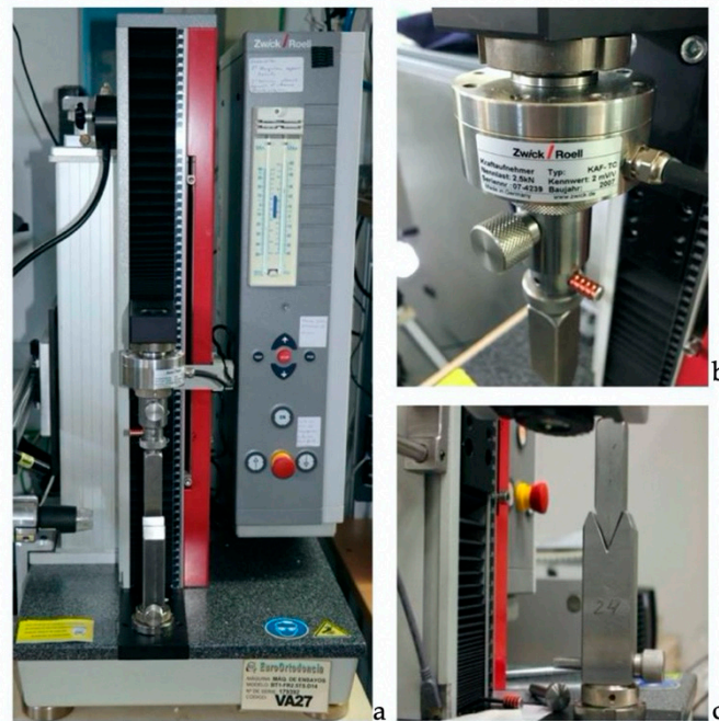
Figure 1. (a) Universal testing machine. The machine consists of (b) a load cell, in charge of measuring pressure and traction; and a motor, in charge of placing the cell at the appropriate distance. In addition, it consists of the (c) supports in charge of simulating 3-point bend test.
