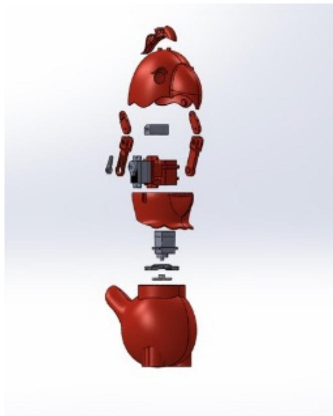
Figure 1. Wearable KiliRo robot—motor positions.
