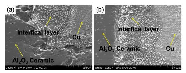
**Figure 2.** SEM images of Cu/Al<sub>2</sub>O<sub>3</sub> composites at bonded temperature 1300 °C: (**a**) without CeO<sub>2</sub> and (**b**) with CeO<sub>2</sub>.
