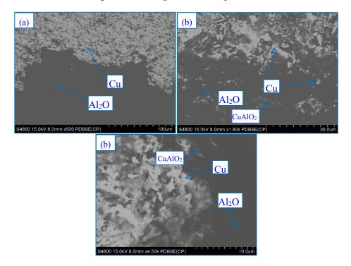
**Figure 8.** Backscattered electron imaging (BSE) images at samples' bonded temperatures: (**a**) without CeO<sub>2</sub> at bonded temperature 1300 °C, (**b**) without CeO<sub>2</sub> at bonded temperature 1500 °C, and (**c**) with CeO<sub>2</sub> at bonded temperature 1300 °C.
