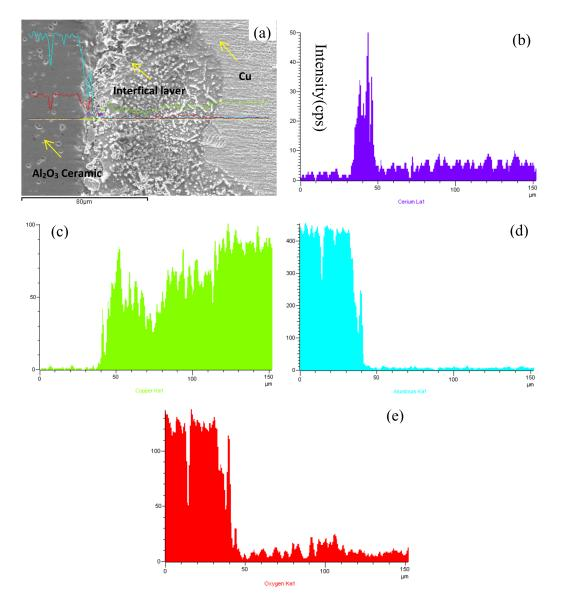
Figure 5. EDS of interface coated with CeO<sub>2</sub>: (a) interface, (b) Ce, (c) Cu, (d) Al, (e) O.
