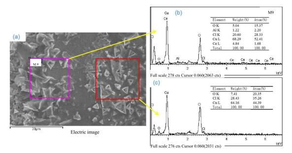
**Figure 10.** SEM images and EDS of interface (Cl is the etched residuum): (**a**) SEM, (**b**) ceramic side, (**c**) Cu side.
