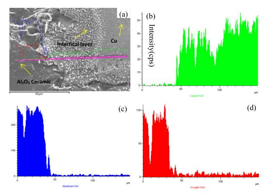
**Figure 4.** Energy-dispersive X-ray spectroscopy (EDS) of Cu/Al<sub>2</sub>O<sub>3</sub> ceramic interface without CeO<sub>2</sub>: (**a**) interface, (**b**) Cu, (**c**) Al, (**d**) O.
