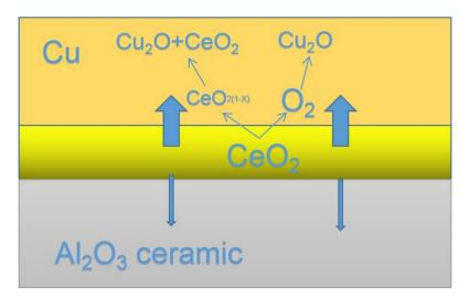
Figure 9. Mechanism of Cu-Cu<sub>2</sub>O-CeO<sub>2</sub> eutectic liquid formation at bonded temperature 1300 °C.
