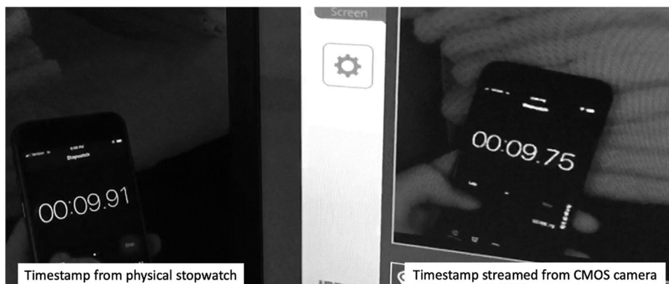
FIGURE 3 A physical stopwatch and streamed view of the stopwatch were captured in the same image. The streaming latency of the complementary metal–oxide–semiconductor (CMOS) camera was calculated as the difference between the timestamp shown on the physical stopwatch and the timestamp that was streamed from the camera.
