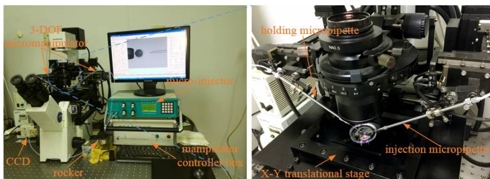
Figure 7. The NK-XMR160 micromanipulation system.
