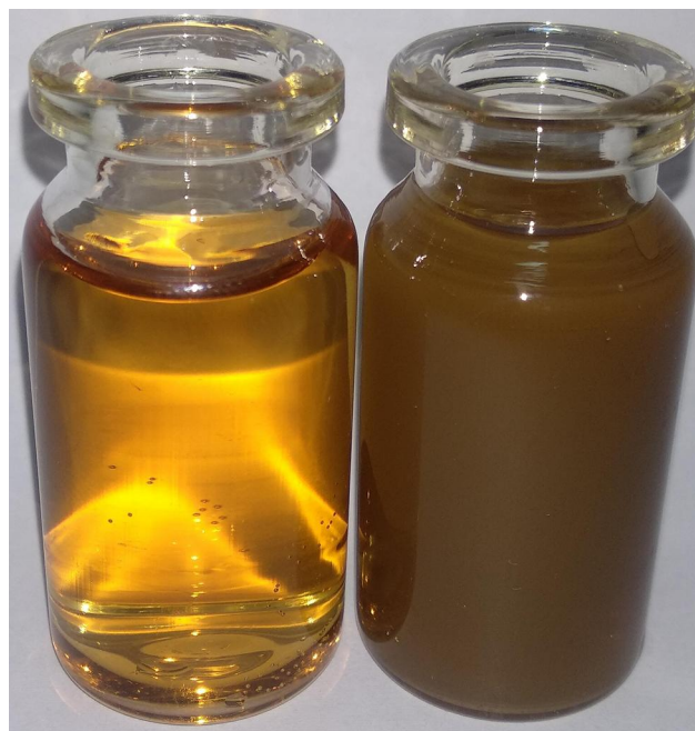
Figure 1 Color change of the reaction solution from light yellow to dark brown after 2 h indicates the formation of PF@AgNPs.
