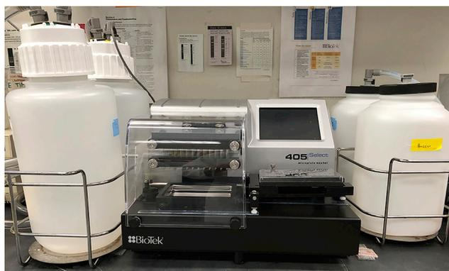
**Figure 1. BioTek 405 TS Microplate Washer**
