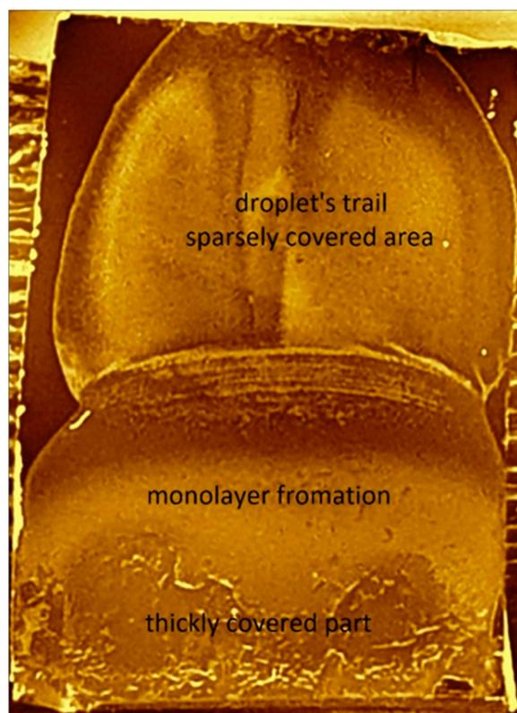
Figure 5. Substrate regions of different coverage formed upon drop casting at an angle.
