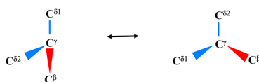
Figure 3. Methyl jumps between two out of the four corners of the carbon tetrahedron, involving an angular change of 110.5^\circ . From the perspective of MOMD, the blue axes denote Z_Q , the red axis denotes Z_M , and \beta_{MQ} is equal to 110.5^\circ .
