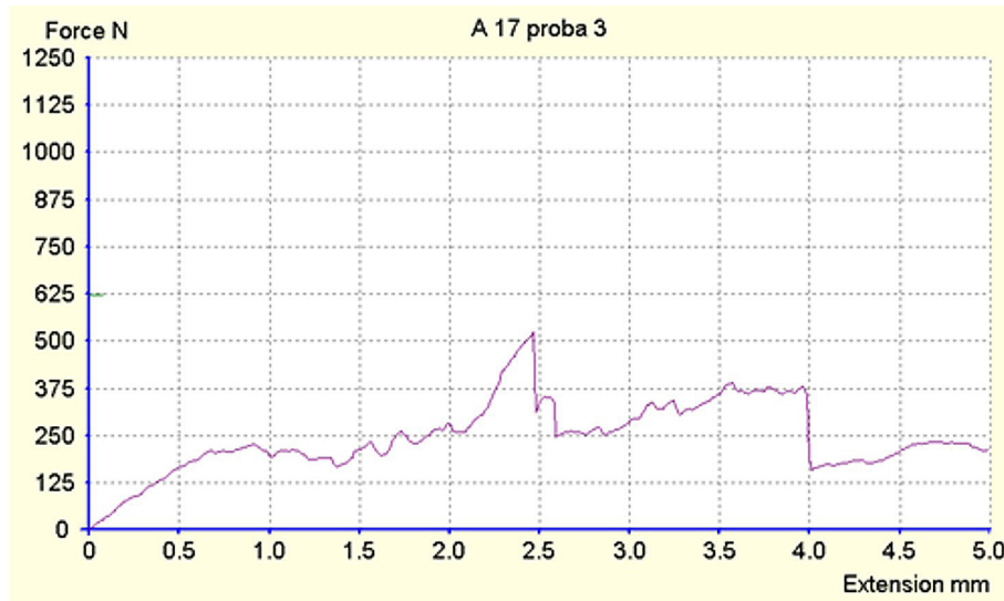
Figure 5. Registration of deformations of the tooth 2.3 restored with Reforpost pivot that remained intact.
