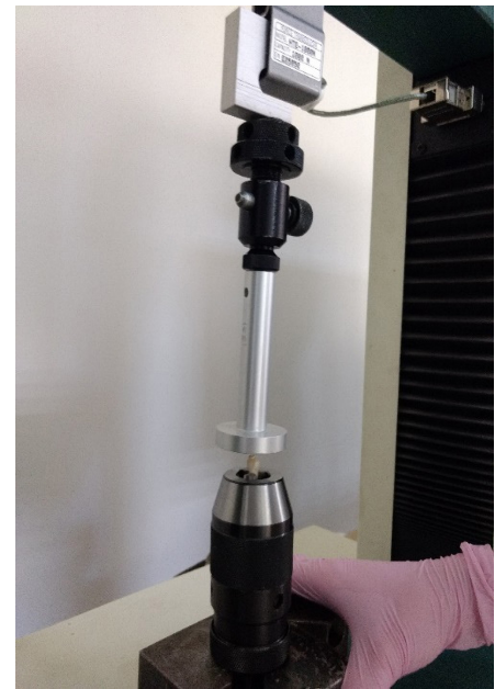
Figure 1. Tooth fixed in unit for mechanical tests using the Hounsfield/Tinius Olsen H1KS tester
